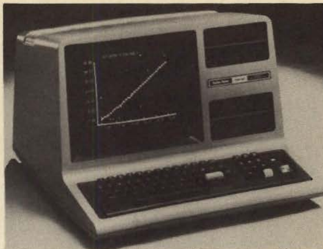
The TRS-80 Model III from Radio Shack is an all-in-one package, with 16K of RAM and a huge variety of software.
