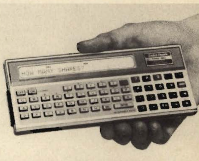
Radio Shack's TRS-80 PC-2 can use cassettes and plug-in memory cartridges; a wide range of software is available.
