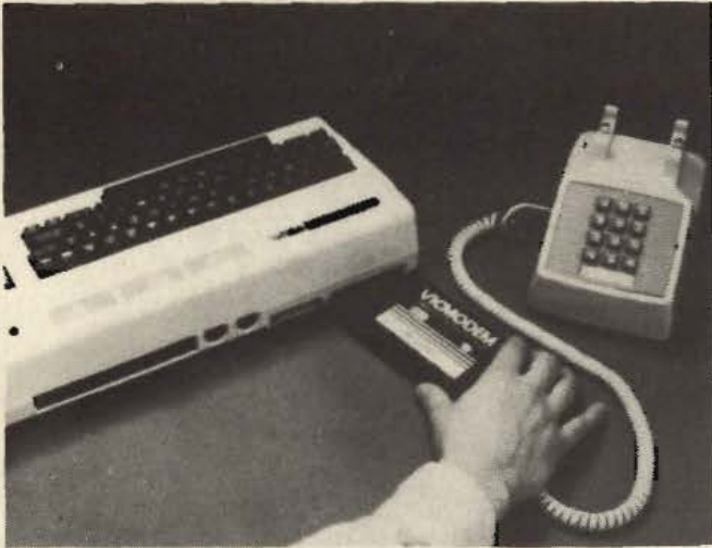
Some modems are made in the form of cartridges, and plug right into your computer. Some even dial for you!
